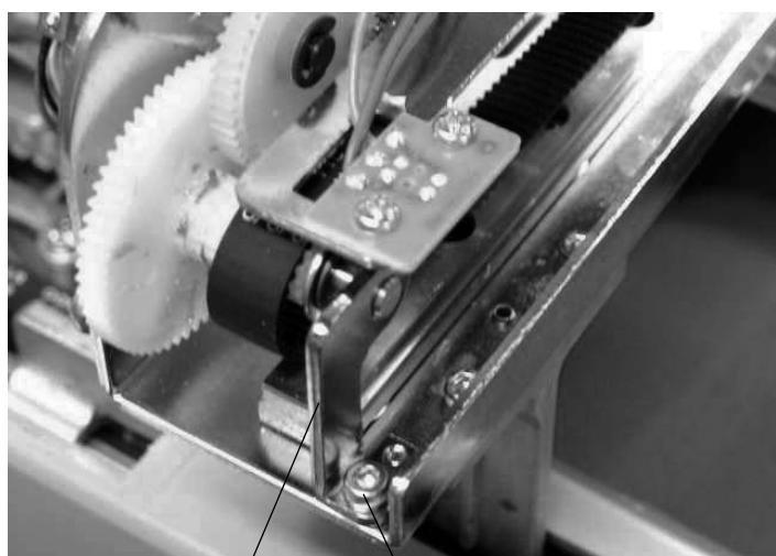
Drive pulley shaft unit
